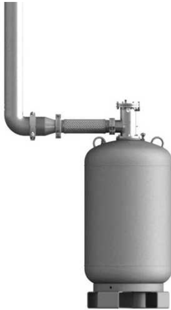
Figure 5.13: Grooved-End Fittings and Horizontal Check Valve Arrangement
