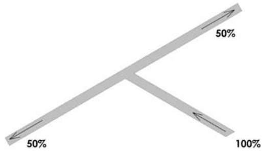
Figure 5.6: Minimum Imbalance for Bull Tee
